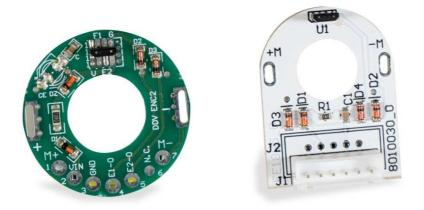
The electromagnetic encoder has been realized for being used as an incremental rotating encoder in more applications. Combined with its own motor, it could be used to control robotic system, the positioning of transport and handling system, as well as in any applications that requires a motor with a speed and position control card.
